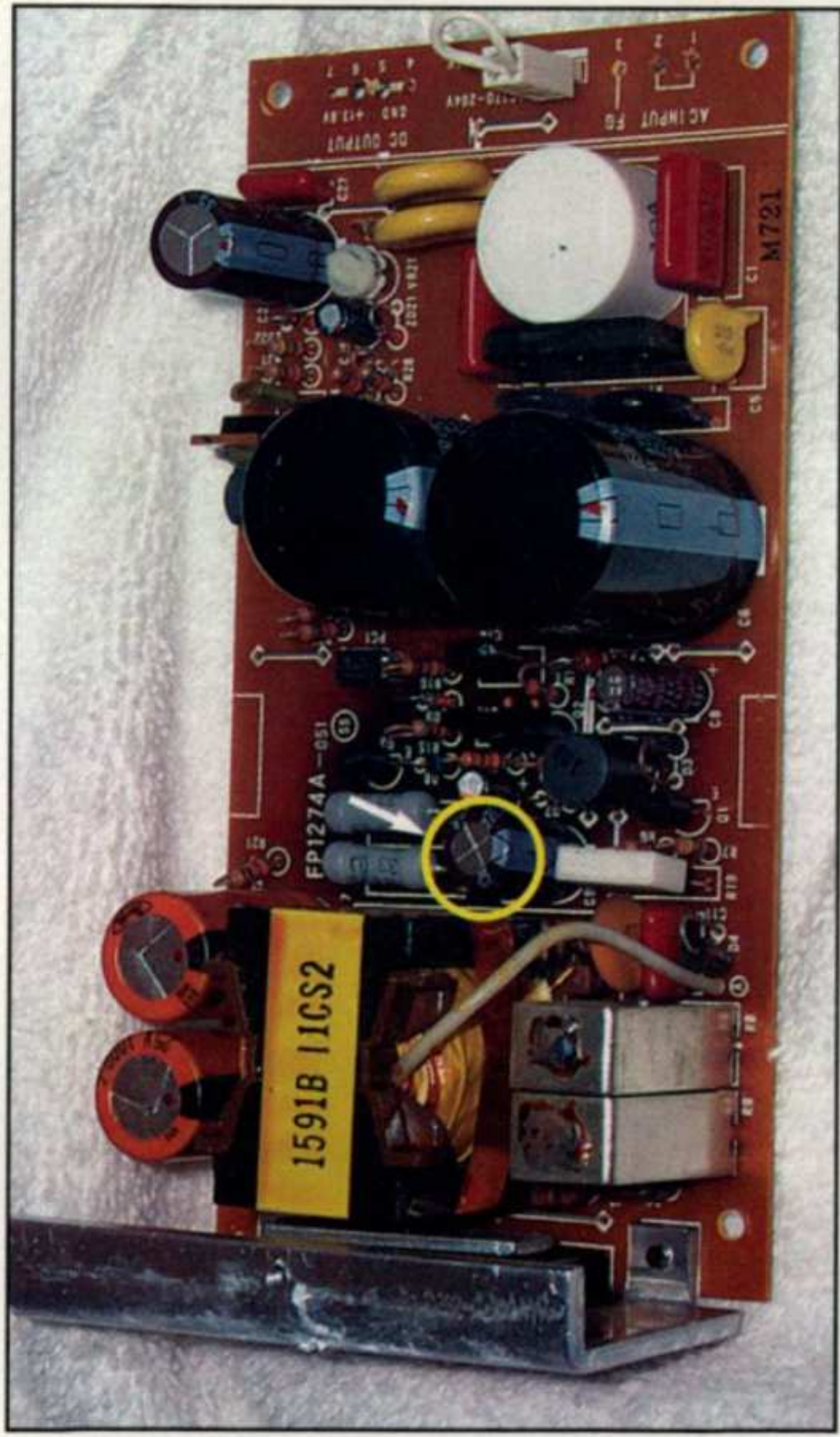
Photo B- The FP127RA stock power supply. Capacitor C9 (highlighted) often fails with age. Sometimes replacing the capacitor will bring the unit back to life. Other times you may need to replace the entire power supply, as explained in this article.
