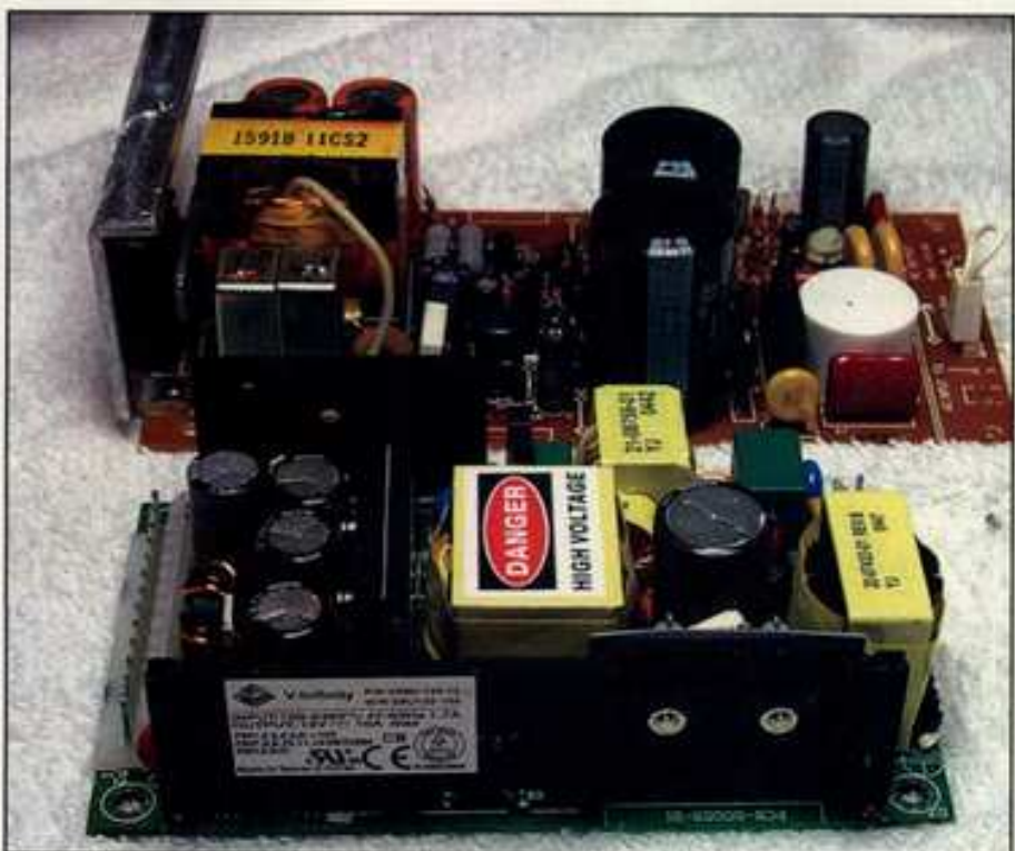
Photo C— The V-Infinity VSBU-120-12, in the foreground, was used as a smaller, quieter, and more reliable replacement for the '736's original FP127RA power supply.
