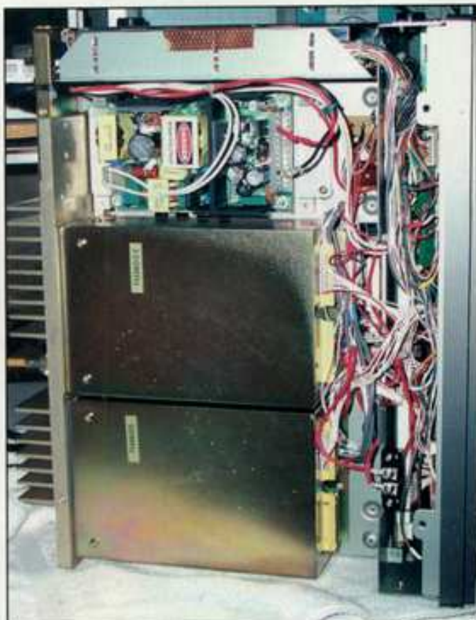
Photo D- The FT-736R with the new switching power supply (top) installed.
